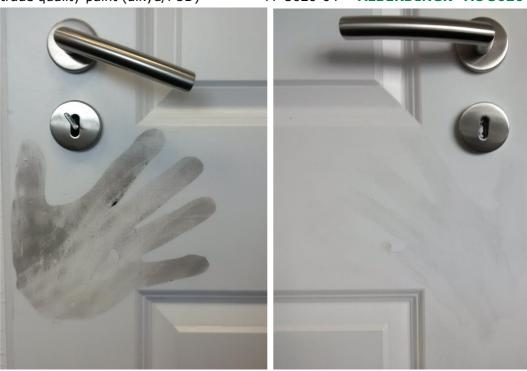
\*16h Alberdingk-fatty acid test which simulates the resistance of the film to human hand fat or hand lotions.
